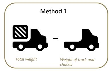
The entire stuffed container is weighed on a certified scale.
