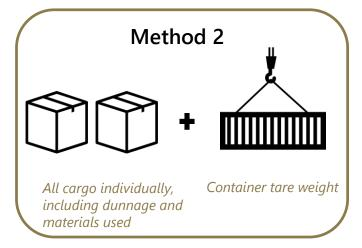
All cargo individually, including dunnage and materials used, is weighted whilst stuffing container, and when the loading is completed, the container tare is added.
